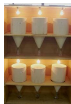
Fig. 4: Extraction of soil fauna. Berlese-Tullgren apparatus.
